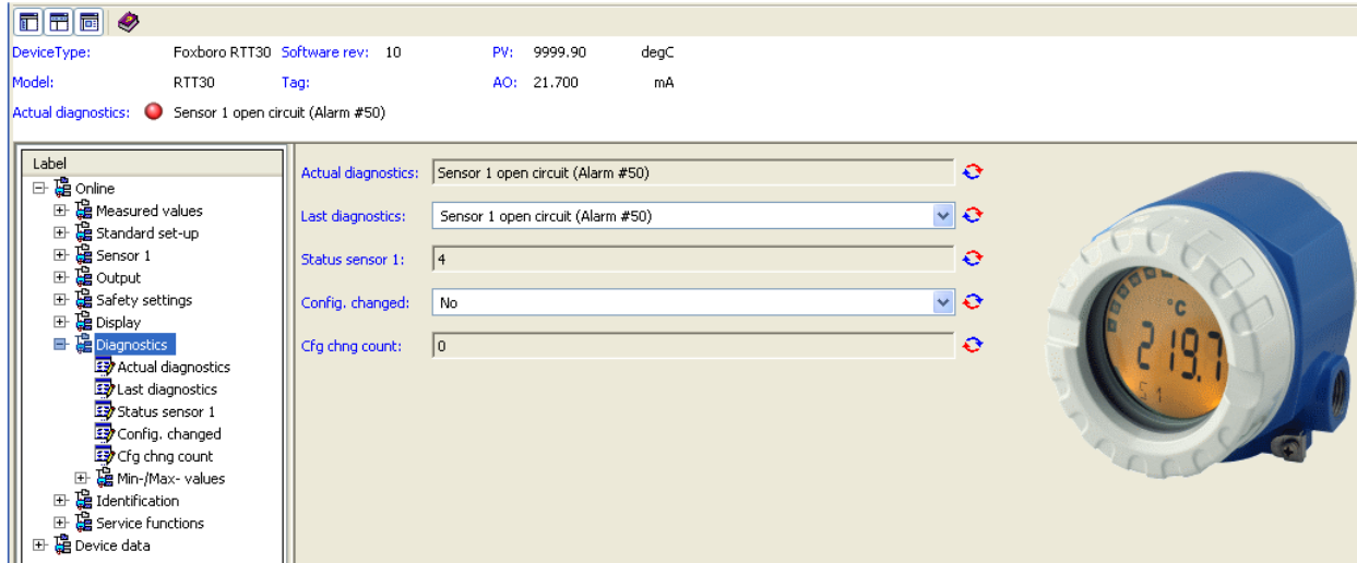
Figure 19. Sample RTT30 Temperature Transmitter Diagnostics Screen
