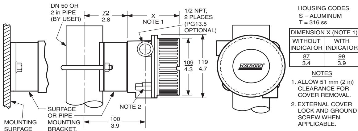
TRANSMITTER WITH INTEGRAL SENSOR (CODES L, M, W, AND Y)
