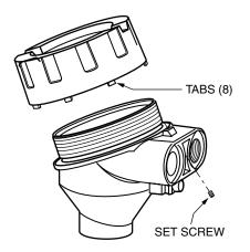
Figure 6. Explosionproof Connection Head Cover Lock
