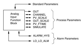
Figure 16. Analog Input Block Parameter Summary
