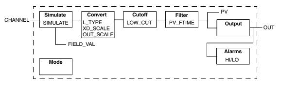
Figure 13. Analog Input Block Schematic
