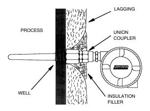
Figure 4. Thermowell Mount (Housing Codes E, F, L, and M)
