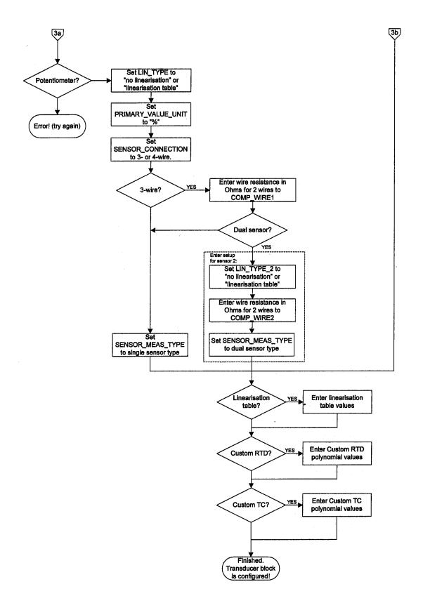
Figure 12. Quick Setup Flowchart (3 of 3)
