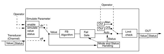
Figure 17. Analog Input Block Simulation, Mode, and Status Diagram
