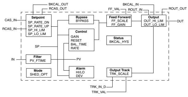
Figure 15. PID Block Schematic
