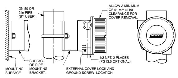
Figure 2. Surface or Pipe Mount with Remote Sensor (Housing Code S and T)
