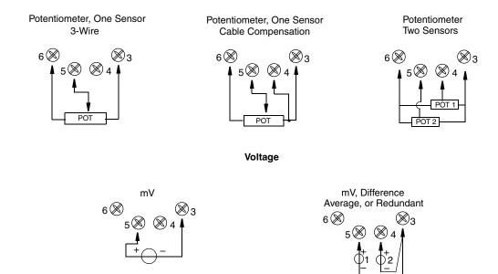
Figure 8. Input Connections (2 of 2)
