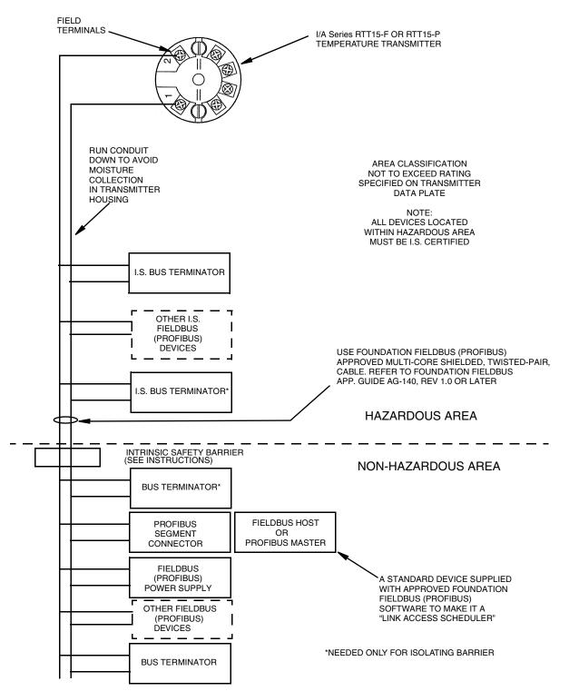
Figure 9. Connecting an RTT15-F or RTT15-P to the FOUNDATION Fieldbus or PROFIBUS
