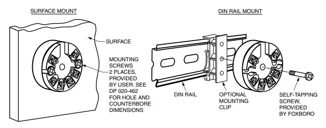
Figure 3. Basic Module Mount (Housing Code B)
