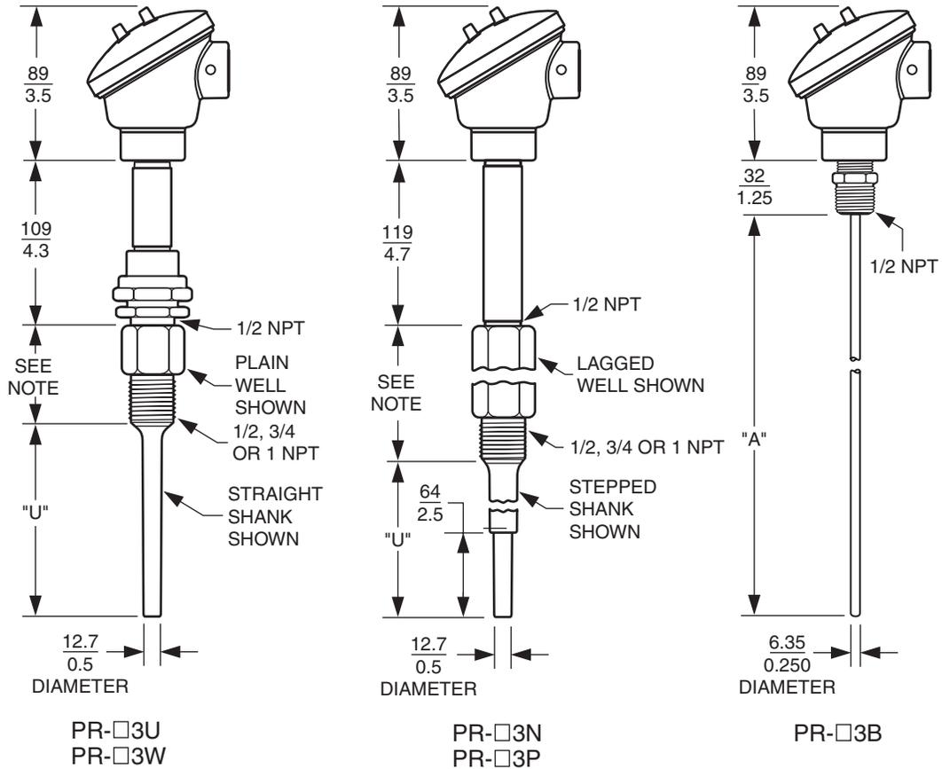
NOTE: T+44 mm (T+1.75 in) FOR THREADED AND WELD-IN THERMOWELLS
