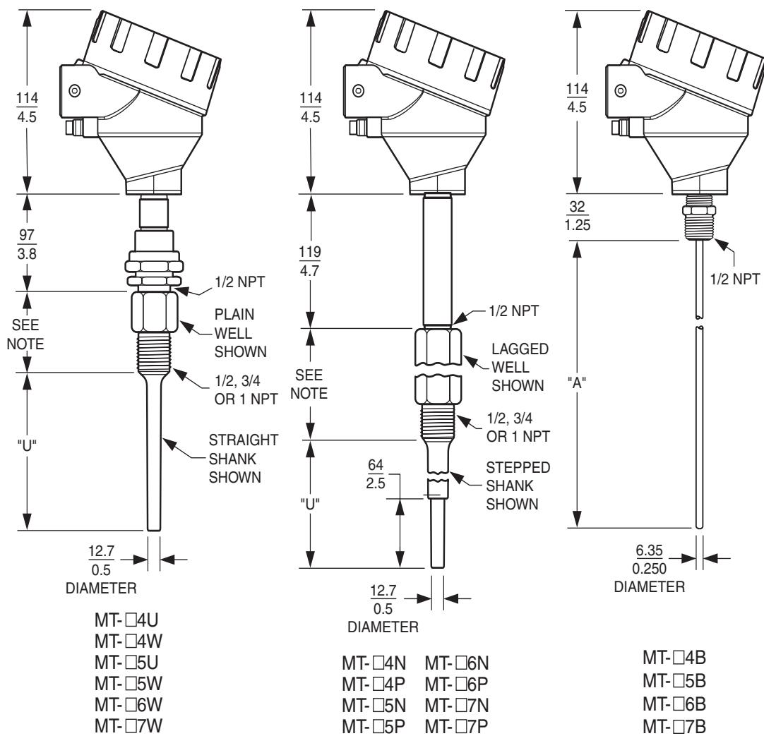
NOTE: T+44 mm (T+1.75 in) FOR THREADED AND WELD-IN THERMOWELLS
