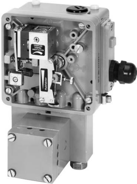
Fig. 4: Single-acting positioner with volume booster
