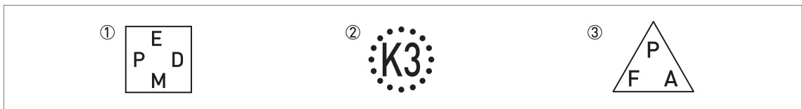
Figure 2-7: Symbols for the supplied gasket material (on the side of the process connection)
