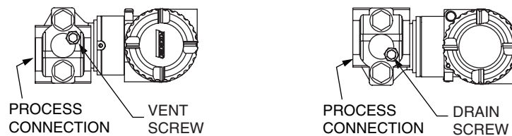
Figure 16. Horizontal Mounting - Cavity Venting and Draining
