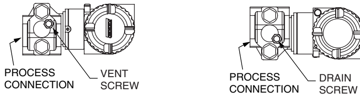
Figure 16. Horizontal Mounting - Cavity Venting and Draining
