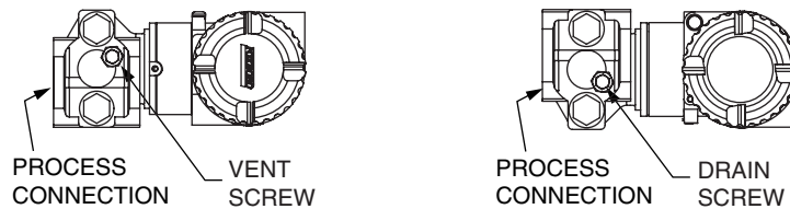
Figure 16. Horizontal Mounting - Cavity Venting and Draining
