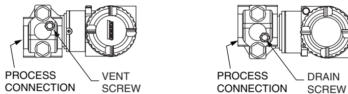
Figure 21. Horizontal Mounting - Cavity Venting and Draining
