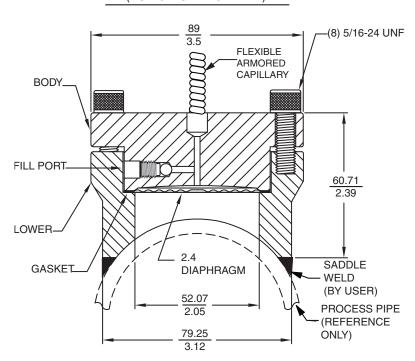
316 ss Flexible Armor lengths between 5 ft (1.5 m) and 50 ft (15.0 m)
