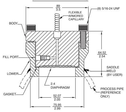
316 ss Flexible Armor lengths between 5 ft (1.5 m) and 50 ft (15.0 m)
