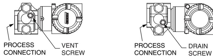
*Figure 17. Horizontal Mounting - Cavity Venting and Draining*
