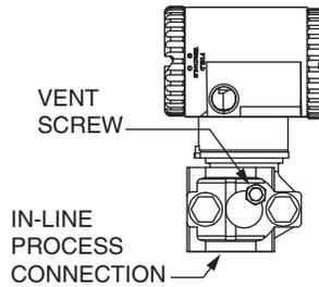
*Figure 17. Horizontal Mounting - Cavity Venting and Draining*
