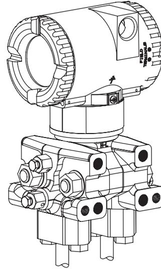
NOTE: MARK INDICATING LOW AND HIGH PRESSURE SIDE OF TRANSMITTER
