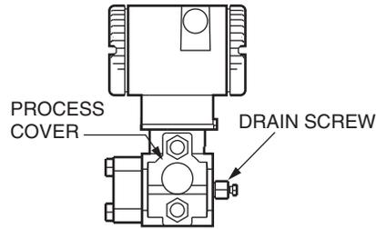
*Figure 14. Vertical Mounting - Cavity Venting*
