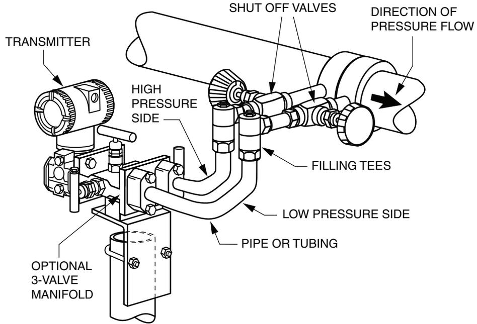
Figure 20. Example of Vertical Process Line Installation
