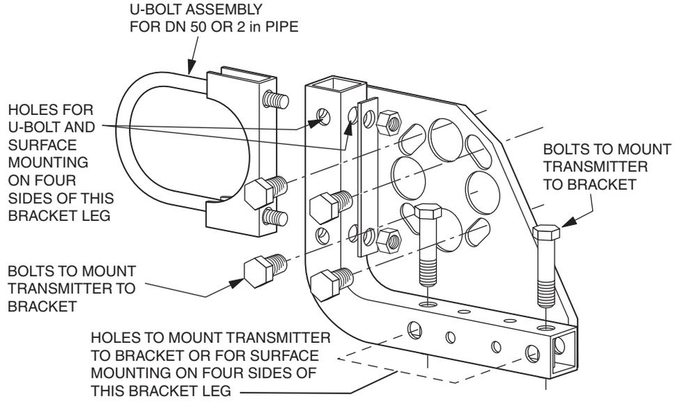
*Figure 10. Mounting a Transmitter with Traditional Structure Using a Universal Bracket*
