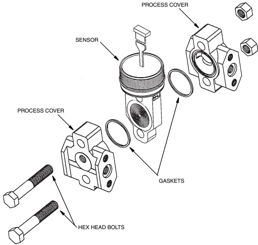
*Figure 39. Replacing the Sensor Assembly (PVDF Inserts)*
