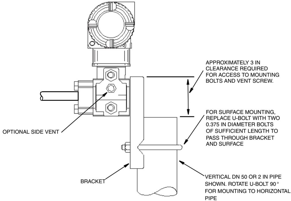
*Figure 8. Examples of Mounting With a Standard Bracket*
