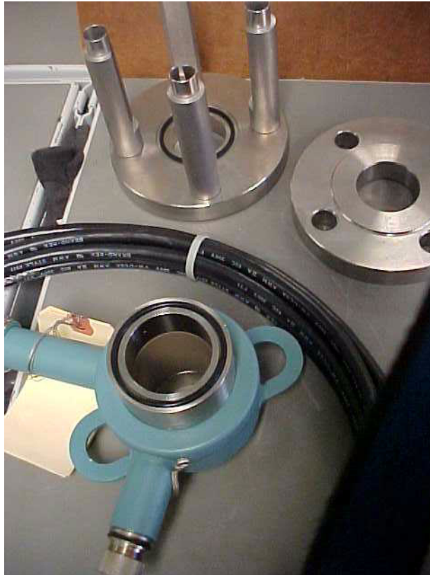
Figure 23. Separation of Flanges from the Toroid Assembly
