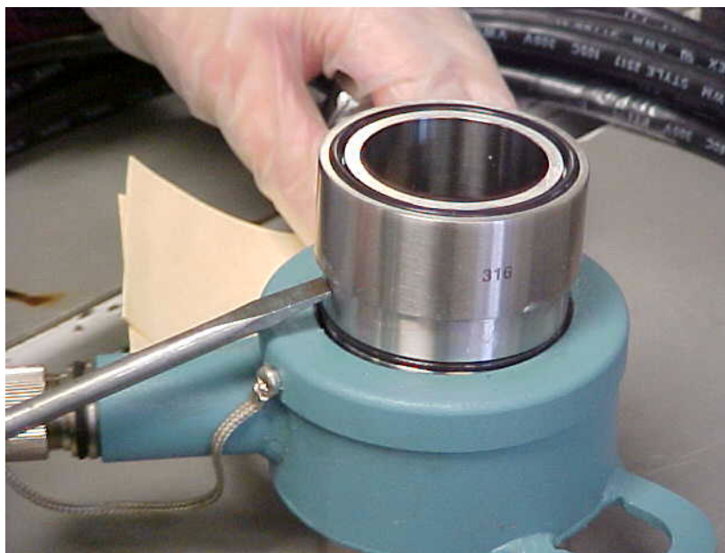
Figure 24. Removal of First Toroid Sleeve from the Toroid Assembly
