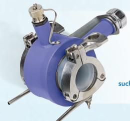
Foxboro's 871FT conductivity sensors are a comprehensive family of flow-through, noninvasive electrodeless assemblies that measure the conductivity of almost any conductive liquid. Featuring a built-in calibration port, the 871FT sensors can be calibrated in-line to improve applications with aggressive chemicals and those in industries such as pharmaceuticals where the process line cannot be broken.
