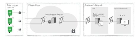
Schneider Electric employs two industry-standard API methods (REST API and SOAP API) for data retrieval from the Schneider Electric Private Cloud. In addition, Schneider Electric provides three data retrieval Agents, which include DNP3, OPC-UA, and CSV, which are traditionally used for SCADA integration.
