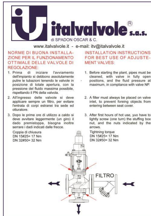
Fig. 3: Back - Proper installation procedure for optimum operation of the GRS/10 2 ways, 3D valves.
