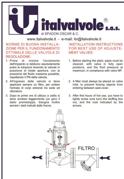
Fig. 3: Back - Proper installation procedure for optimum operation of the GRS/10 2 ways, 3D valves.
