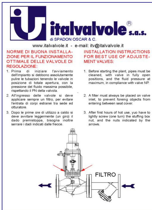
Fig. 3: Back - Proper installation procedure for optimum operation of the GRS/10 2 ways, 3D valves.
