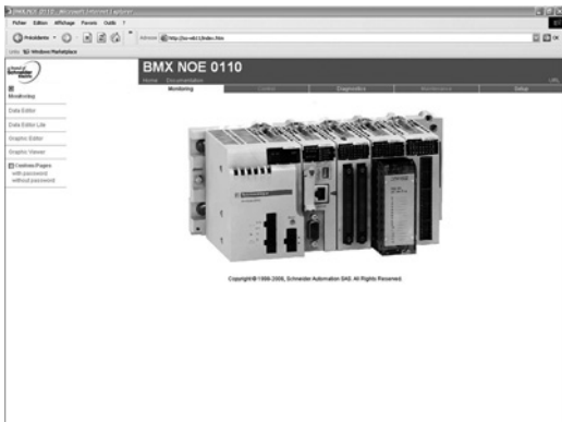
Modicon M340 hardware configuration
