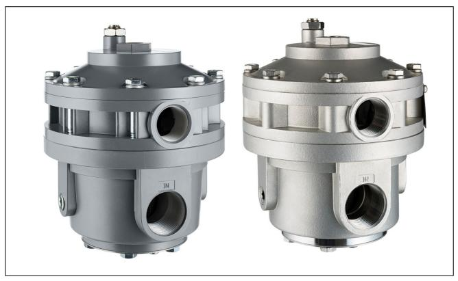
The VBS300 Volume Booster Series is designed to operate pneumatic valve actuators via a valve positioner. It is recommended for large actuators to reduce positioning time. Volume boosters with Cv 5 and pneumatic connection 1", for remote mounting. VBS300 in Aluminum, VBS310 in Stainless Steel 316. The bypass valve is used to adjust dynamic response to provide stable operation over a wide range of actuator sizes.
