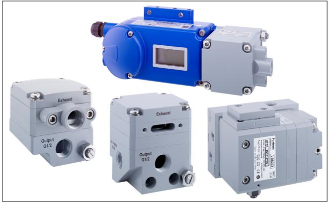
The VBS200 Volume Booster Series is designed to operate pneumatic valve actuators via a valve positioner. It is recommended for large actuators to reduce positioning time. The bypass valve is used to adjust dynamic response to provide stable operation over a wide range of actuator sizes.
