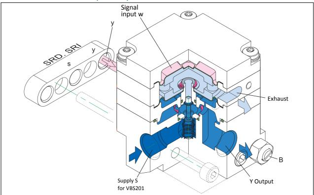
Output y of Positioner is connected to chamber w of Booster. Bypass-screw B controls the flow between input w and output Y of Booster. SRD / SRI supply is connected at the rear side of the VBS201 housing and is forwarded to the positioner.
