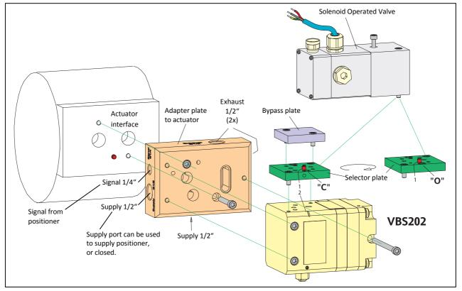
Note: The both Supply air 1/2" connections are directly connected to each other on the Adapter plate. The connection left hand Supply air 1/2" is usually looped through to supply the upstream position control. If the supply air pressure for the actuator is higher than for the positioner, an air supply station must reduce the pressure for the positioner to a permissible value.
