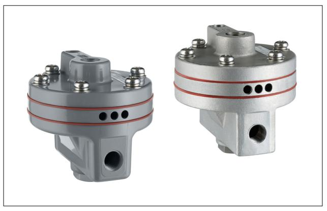
The VBS100 Volume Booster Series is designed to operate pneumatic valve actuators via a valve positioner. It is recommended for large actuators to reduce positioning time. The bypass valve is used to adjust dynamic response to provide stable operation over a wide range of actuator sizes.
