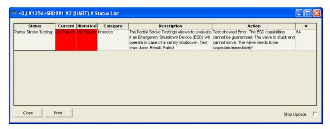
Moreover this information can be stored and read by a condition monitoring system like Avantis CM (Conditioning Monitoring). The Avantis CM will notify key personnel by email (for example, whenever a PST bad status occurs) and recommend a list of corrective actions.
