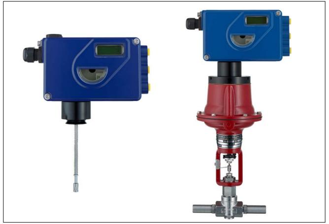
This version is designed for direct mounting on top of small actuators without yoke - solution for actuators up to 50 mm stroke. Instead of the rotary potentiometer, a linear pot is used that feeds back the actual position of the actuator.
