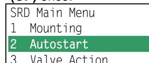
Now press keys (UP)+(DOWN) simultaneously to enter menu 'Autostart'.
