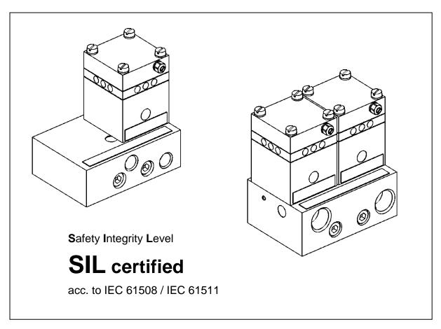
The booster relays LEXG-Fx/Xx and LEXG-Hx/Zx are used in combination with the Intelligent Positioner SRD991 or the universal Positioner SRD960 to operate pneumatic valve actuators from control systems or electrical controllers that are consistent with the special safety requirements according to IEC 61508 / IEC 61511-1. The considered safety related application of the positioner for pneumatic actuators is as a shutdown device with fail-safe single-acting (spring return) actuation.
