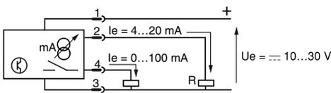
$R_{max.} < 800 \Omega$  ( $U_e = 24 V$ ),  $< 300 \Omega$  ( $U_e = 12 V$ )
