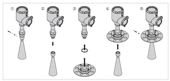
Figure 3-16: Device with a metallic horn antenna
