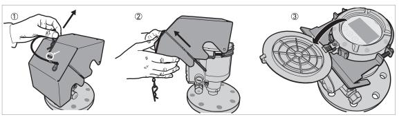
Figure 3-22: How to open the weather protection
