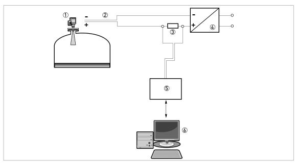
Figure 4-8: Point-to-point connection (non-Ex)
