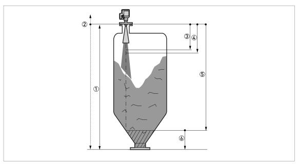
Figure 6-7: Distance measurement
