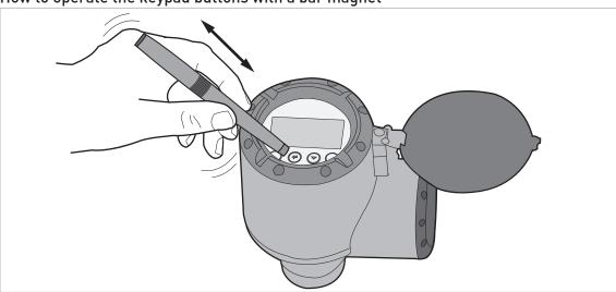
How to operate the keypad buttons with a bar magnet
