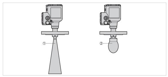
Figure 2-2: Types of antenna
