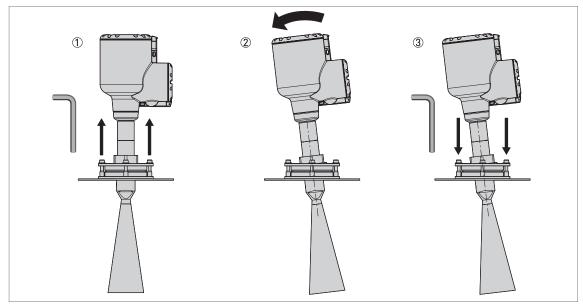
Figure 3-18: How to tilt the device
