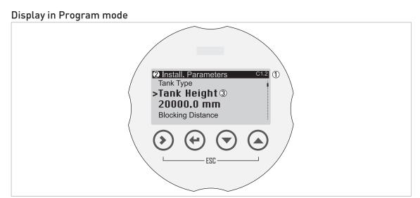
Figure 5-2: Display screen layout in Program mode
