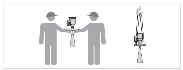
Figure 3-2: How to lift the device
