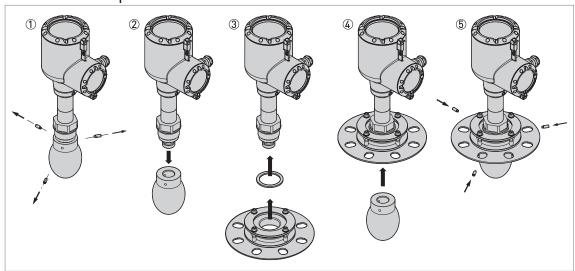
Figure 3-17: Device with a Drop antenna
