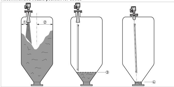
Figure 3-4: Recommended nozzle position for solids
