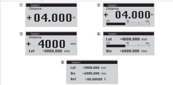
Figure 6-1: Measurement data options in Normal mode
