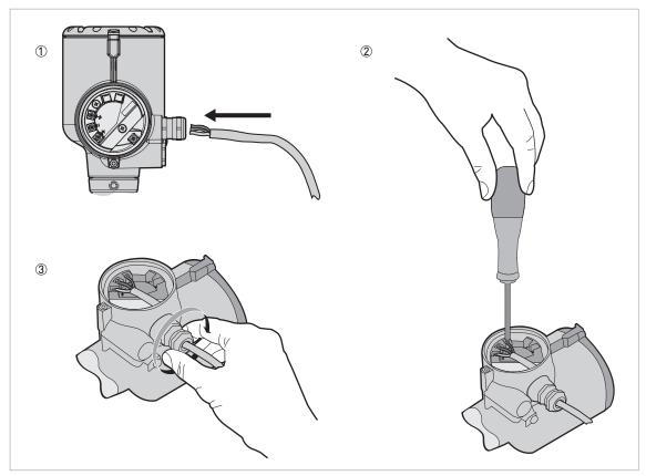
Figure 4-3: Procedure for electrical installation
