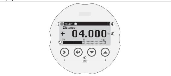
Figure 5-1: Display screen layout in Normal mode (measurement data)
