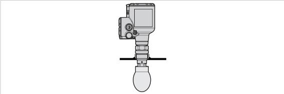
Figure 3-12: Threaded connections: installation procedure
