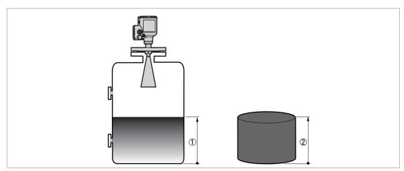
Figure 10-5: Measurement definitions: level
