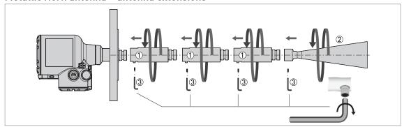
Figure 3-14: Metallic Horn antenna – how to attach antenna extensions
