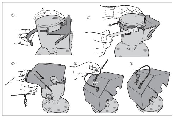
Figure 3-21: Installation of the weather protection
