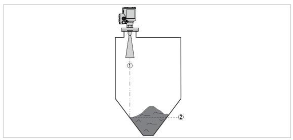
Figure 3-7: Tanks with dish-shaped or conical bottoms
