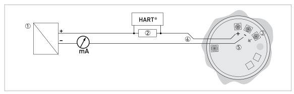
Figure 4-6: Electrical connections for non-Ex devices
