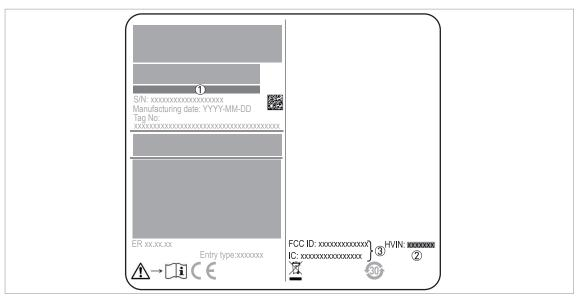
Figure 1-2: U.S.A. and Canada: radio approval information on the nameplate
