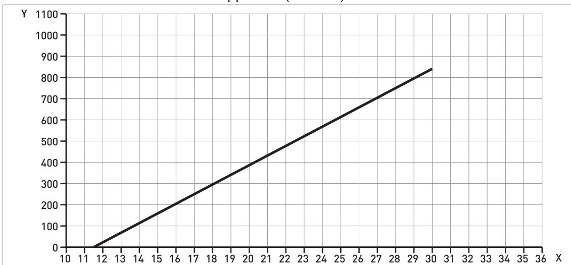
Figure 3-8: Minimum power supply voltage for an output of 22 mA at the terminal (Non-Ex and Hazardous Location approval (Ex i / IS))
