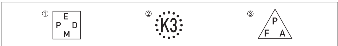
Figure 2-3: Symbols for the supplied gasket material (on the side of the process connection)
