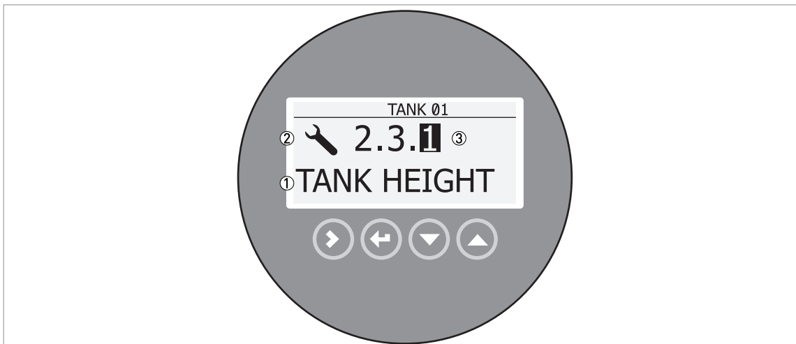
Figure 5-2: Local display screen layout in configuration mode
