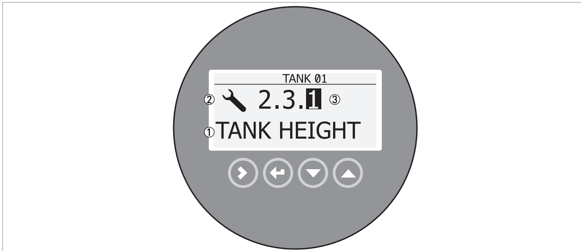
Figure 6-1: Local display screen layout in configuration mode
