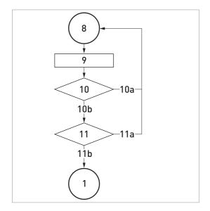
8 Error mode state 9 Current output (error value) 10 Is the parameter set for the current output 10a No. The parameter set for the current output is incorrect. 10b Yes. The parameter set for the current output is correct 11 Is a new correct measurement available? No. A correct measurement is not available. 11a Yes. A correct measurement is available. 11b Initial state (new measurement) 1
