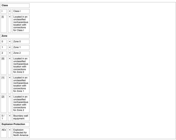
"Division" equipment with supplemental "Zone" marking as permitted by Section 505-9 (c) (1) of the NEC does NOT show the "AEx" designation, see Example 2.
