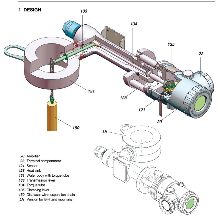
For left-sided mounting all inside parts are arranged in inversed manner.
