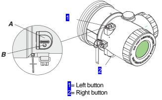
After shifting the key protection cap **A**, insert screw driver or pin ( $\emptyset < 3$  mm) into hole **B** and press down to the second pressure point.
