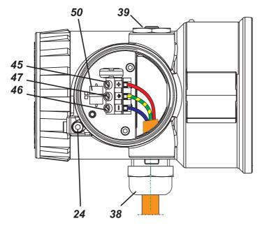
Guide **cable** through cable gland **38** from the bottom; observe especially the shielding.
