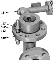
In order to make mounting easier, mounting bracket **132** is secured with a stud **142** to connecting flange **140**. It is advisable to preassemble a stud by screwing a nut **143** onto thread.
