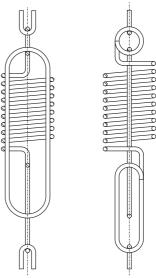
It is hooked onto the suspension chain of the displacer in place of 7 chain links (105 mm). This spring is specially matched to the resonance frequency of the displacer and is made of stainless steel 1.4310 (operating temperature up to 250 °C) or Hastelloy C (operating temperature up to 350 °C).
