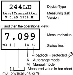
The operational view is the display in normal operation.
