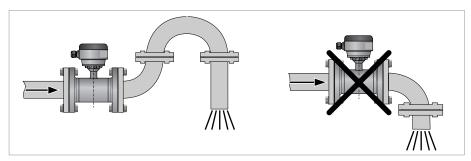
Figure 3-9: Installation in front of an open discharge
