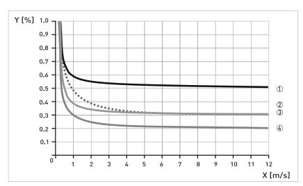
Figure 6-2: Flow velocity vs. accuracy
