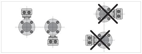
Figure 3-15: Mounting position
