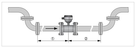
Figure 3-4: Recommended inlet and outlet
