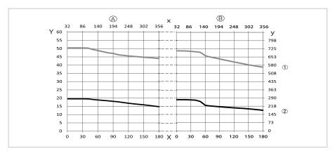
Figure 6-4: Pressure derating; ANSI B16.5
