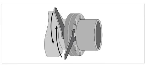
Figure 3-16: Tightening of bolts
