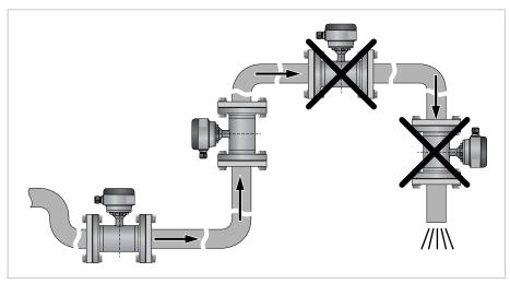
Figure 3-7: Installation in bending pipes (90°)
