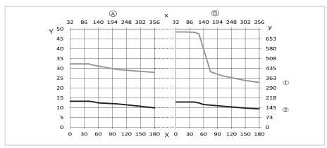
Figure 6-5: Pressure derating; JIS B2220
