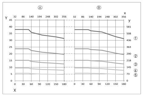
Figure 6-3: Pressure derating; EN 1092-1
