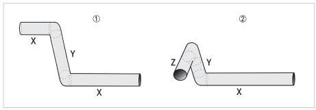
Figure 3-5: 2 and/or 3 dimensional bends upstream of the flowmeter
