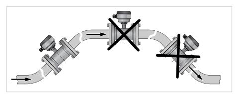
Figure 3-8: Installation in bending pipes (45°)
