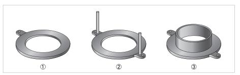
Figure 4-2: Different types of grounding rings
