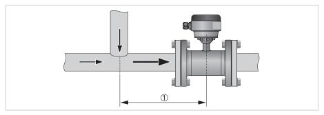
Figure 3-6: Distance behind a T-section
