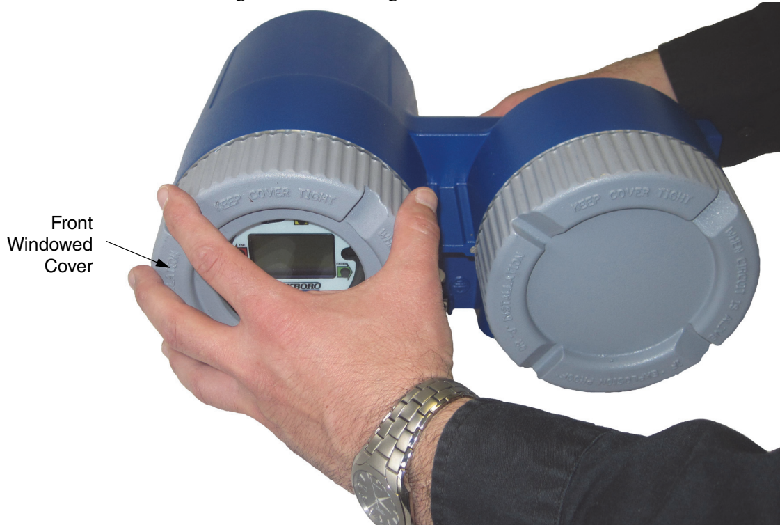
Figure 51. Removing the Front Windowed Cover
