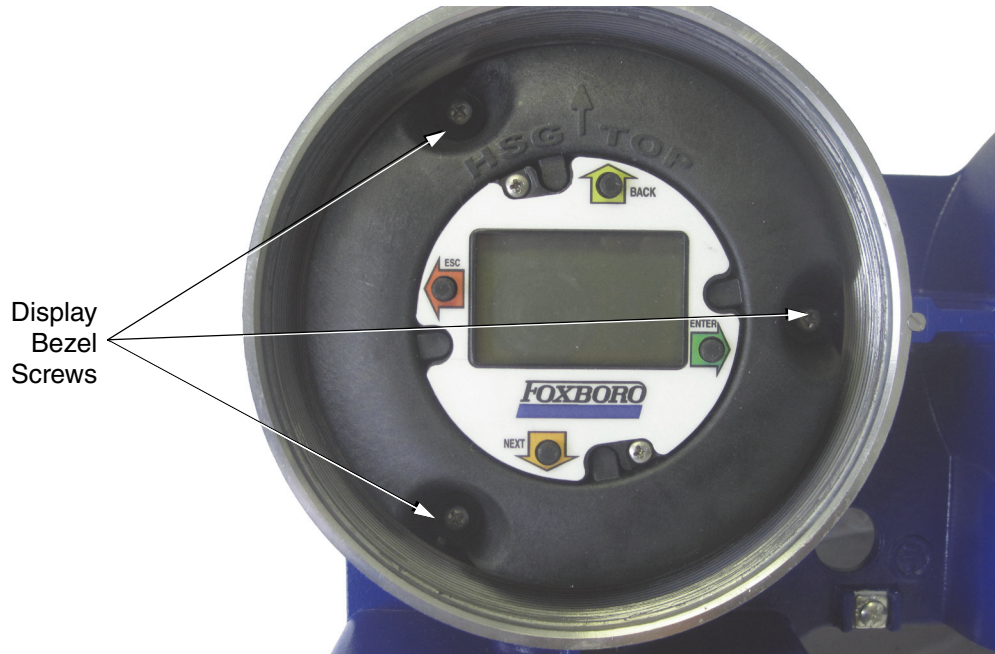
Figure 52. Loosening the Display Bezel Screws
