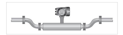
Flexible connections can be used but because of the high flow rates associated with large diameter meters, it is recommended that flexible connections are not used on meters larger than size 80.
