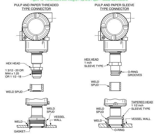
Figure 43. Transmitters with Integral Pulp and Paper Process Connections
