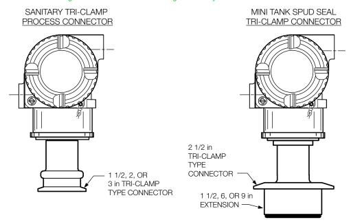
Figure 41. Transmitters with Integral Sanitary Process Connections
