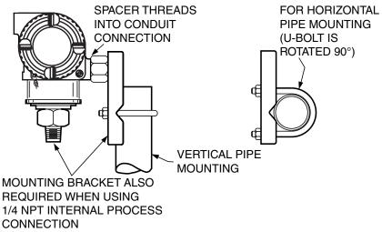
Figure 21. Mounting Bracket Sets -M7 and -M8 for IAP10S/IGP10S Flameproof Transmitters
