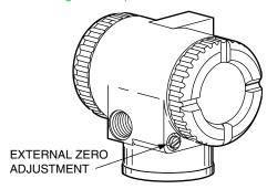
External Zero Adjustment cannot be used with Electronics Versions -A (Analog) and -V (Low Power).
