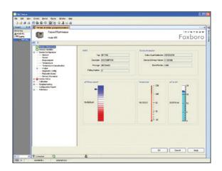
**HART DTM:** A time-saving HART Device Type Manager (DTM) simplifies configuration and troubleshooting, and provides trend graph capabilities.
