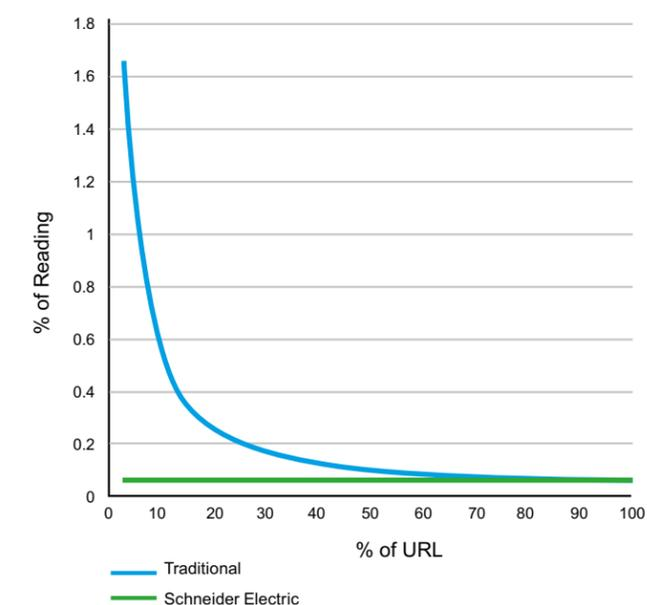
Schneider Electric Pressure Advanced and Premium Transmitters maintain the same percentage of reading accuracy from 100% up to 4% of URL. Traditional transmitters begin to degrade at a much higher percentage.
